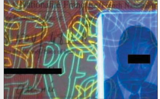
Fluorescent security features viewed under incident UV light.
