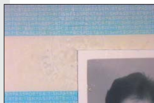
Coaxial lighting reveals retro reflective security patterns.
