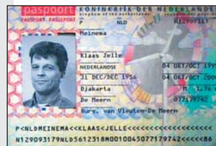
Fluorescent security features viewed under incident UV light.
