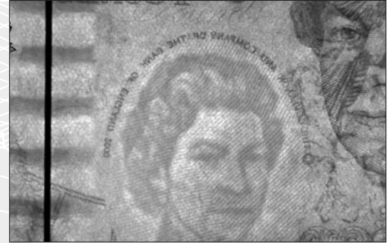
Watermarks and security threads viewed with white transmitted light.
